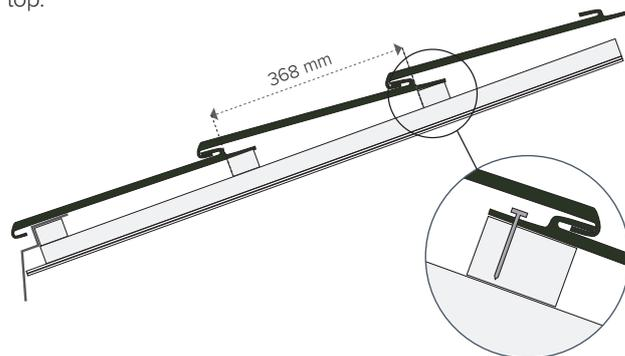
The panels are placed onto deck or battens spaced 14.5" or 368 mm.
