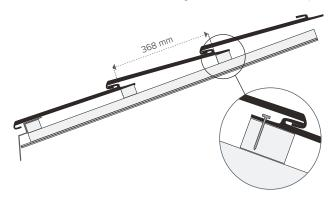
The panels are placed onto deck or battens spaced 14.5" or 368 mm.
